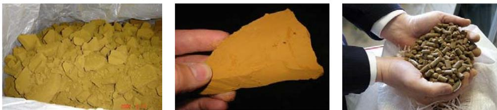
Figure 1: Lignin produced in the demonstration plant of Bäckhammar – filter cake and lignin pellets
